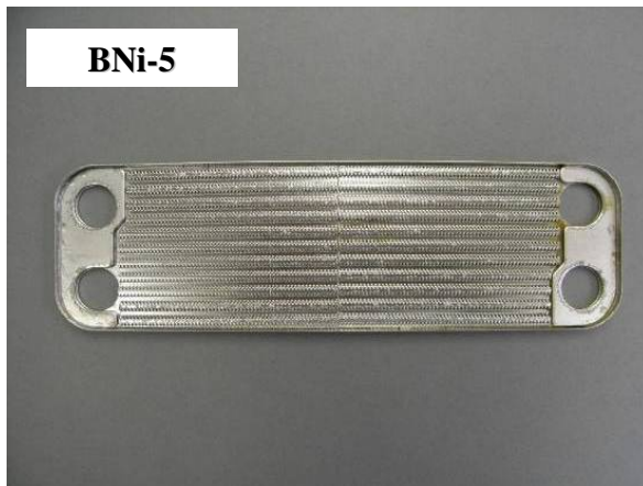
Figure 5 Appearance of after the salt splay test.
